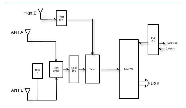
As can be seen, the principal difference is that the RSPduo contains two tuners as opposed to the RSP2 which has a single tuner and switched antenna ports.
