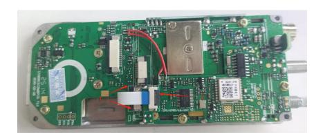
13. ①When welding the RF coaxial cable of the GPS ceramic active antenna, pay attention to the welding speed. The ground wire should not be short-circuited or falsely welded. If the welding is not good, the GPS signal received later will be poor or no satellite will be received; ②Fix the foam on the side of the GPS antenna; ③Insulating paper is attached to the AM antenna head of the expansion board and the pad of the row seat to prevent short circuit with the GPS antenna;
