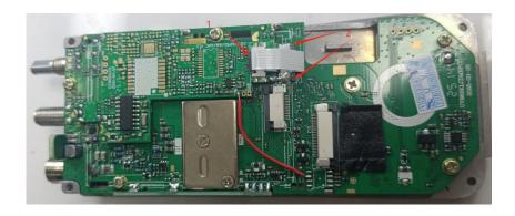
9. ①Solder the electronic connection wires of the expansion board with ferrochrome; ②③④⑤Then use chromite welding to remove the fixed welding points of the expansion plate; ⑥Then, solder the AM antenna head and the socket pads of the expansion board with ferrochrome. Remove the expansion board and solder the excess tin slag on the surface with ferrochrome;
