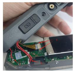
18. Insert the aluminum shell at an Angle of about 30 degrees into the face shell, and place the keyboard flexible flat cable, grounding wire and charging flat cable inside properly to prevent them from being pressed after the shell is installed. Before packing the case, make sure to clean the dust off the surface of the display screen and the lenses first.
