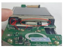
16. ①Align the conductive shielding cloth with half of the FPC socket on the keyboard board and start pasting along the flexible flat cable tape of the earphone PCB to prevent electromagnetic interference; ②Be careful not to short-circuit the FPC pin and the MIC microphone pad.
