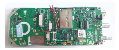
11. ①Solder the AM antenna head and the socket pad with ferrochrome; ②③Then solder the electronic connection wires of the expansion board onto the application pads of the main board. Be careful not to weld in reverse, short-circuit or falsely weld;
