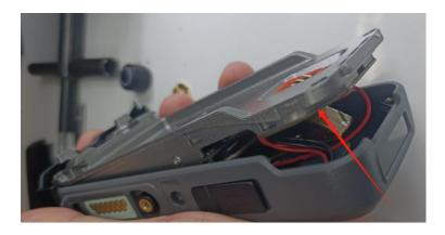
6. ① Unplug the TYPE-C charging ribbon cable; ② Weld the grounding wire welding point with ferrochrome. ③ Then, use tweezers to gently push out the ears on both sides of the FPC power socket, pull out the keyboard and connect the flexible power cable.
