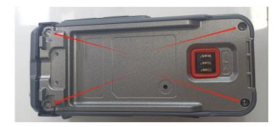
5. After the face shell and the aluminum shell are separated, slowly pull out the aluminum shell;
