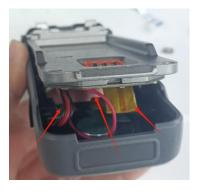
19. Tighten the screws at the front and back of the fixed aluminum shell, Before locking the screws, check if there is any key jamming on the side buttons. If there is, the machine at the back cannot be turned on.
