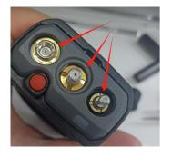
3. Remove the screws that fix the rear shell;
