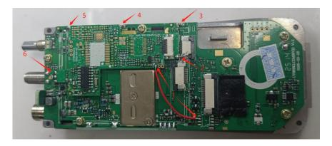
10. Install the expansion board with GPS function into the corresponding position, ①First, fix a point when welding with ferrochrome. Then, adjust the position of the expansion plate to ensure it does not extend beyond the aluminum shell; ②③④⑤use ferrochrome to weld the fixed solder joints of the expansion plate well;
