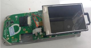
8. ①The tweezers lift the flip cover of the FPC row seat on the expansion board and pull out the end connected to the flexible flat cable. ②Then, use tweezers to gently push the ears on both sides of the FPC socket of the motherboard outward, pull out the connection end of the flexible flat cable, and remove 35mm of the FFC connection flexible flat cable from the other end.
