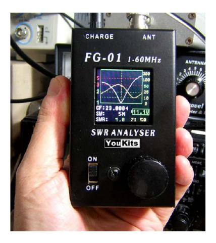
The FG-01 antenna analyzer can be powered by an optional internal battery **TEN-TEC part number R9411**: consisting of a 18650 Lithium battery pack with a built in protection circuit, the standard charging voltage is 11.1Vdc. If powered from an external supply you must use a stable DC power supply with 10-12.8Vdc, @ 500ma. Do not use a power supply greater then 12.8Vdc
