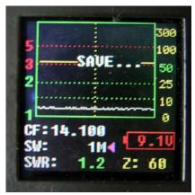
CF or (Center frequency), the center vertical line on the display. This is typically the center frequency of the antenna you are wishing to analyze.
