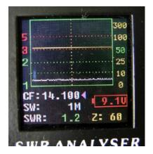
Battery indicator turns red when the battery voltage is lower than 9.5Vdc, you must charge the battery immediately or damage to the battery will occur!
